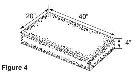
If you use a concrete bag mix, use the mix for maximum strength. An average 80 pound bag of concrete mix will make approximately 2/3 of a cubic foot of concrete.
